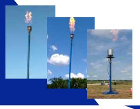
Our flares/tips can achieve a 99.5% destruction rate efficiency which exceeds the EPA's 98.5% requirement under
